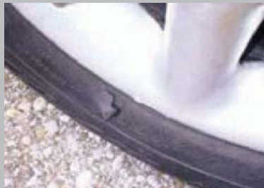
Tyres with impact damage e.g. 'kerbing', bald tyres and those below 2mm tread depth are unacceptable.
